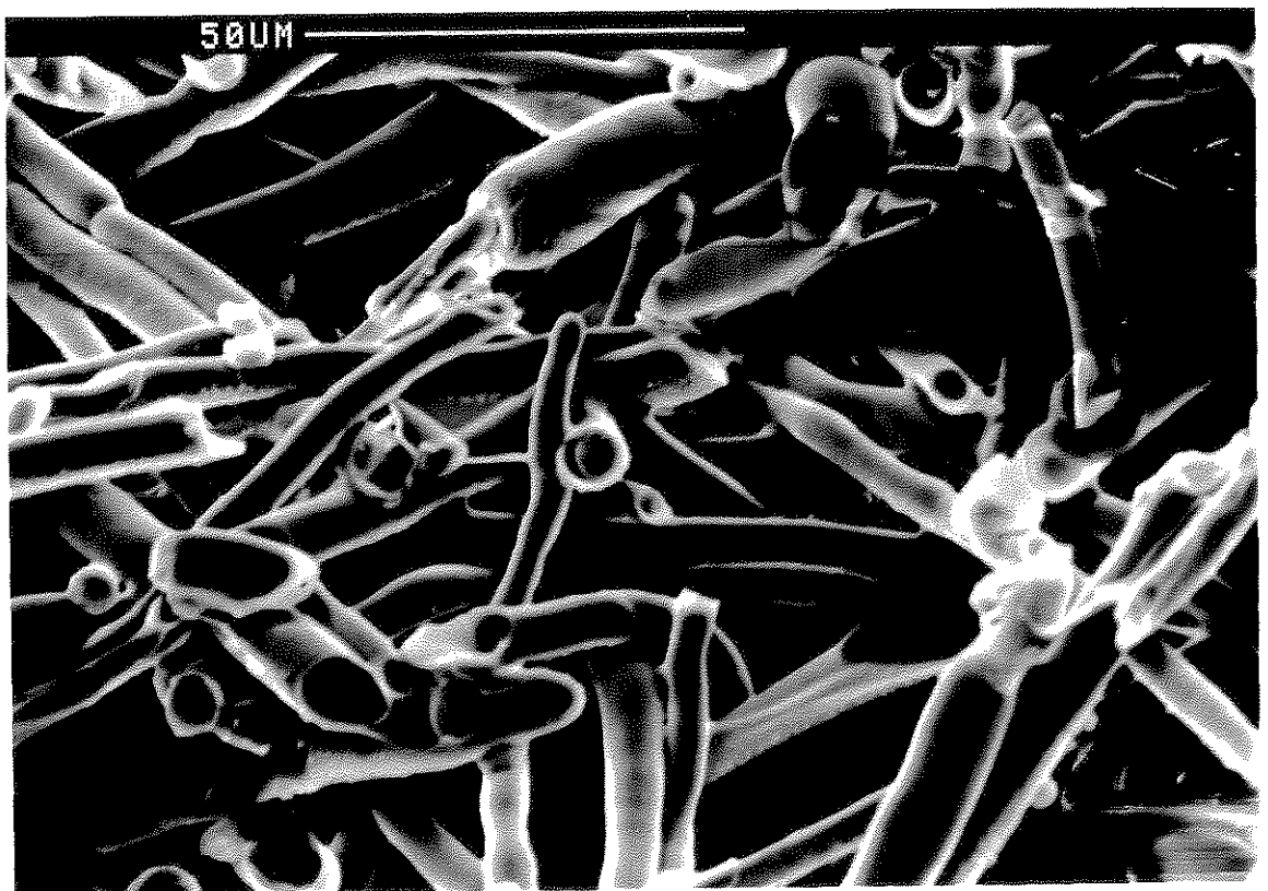
Photo VII.10: Scanning electron micrograph showing intact hyphae underneath the compressed surface.
